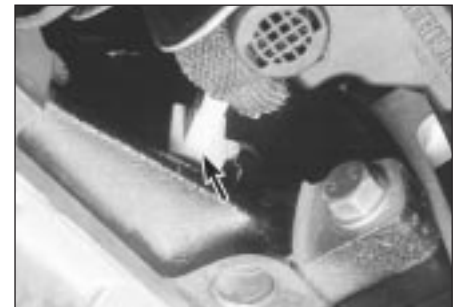
9.4 Location of crankshaft speed/position sensor - connector arrowed - in front of cylinder block/crankcase
