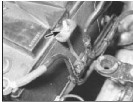
2.2A Unscrew hold-down nuts (one of two arrowed) . . .
