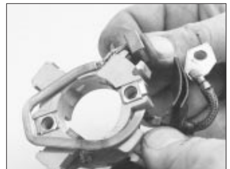
17.2I . . . note how the bus bar is engaged on the brushbox before removing it
