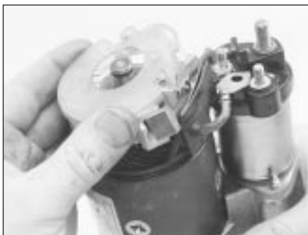
17.2G . . . lift off the plastic insulating plate . . .
