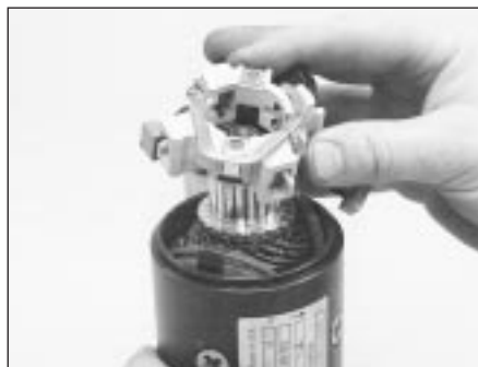
17.2H . . . remove the brushbox and remove the positive brushes complete with the bus bar . . .
