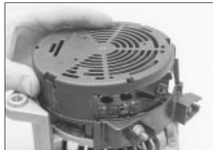
13.2 Renewing voltage regulator/brush holder - Bosch alternator. Remove three screws and withdraw end cover . . .
