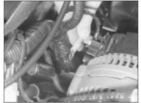
12.3 Disconnecting alternator wiring
