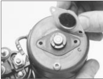
17.2A Remove the two screws to release the end cap. Withdraw the gasket and prise out the C-clip, noting any shims fitted to control armature endfloat . . .
