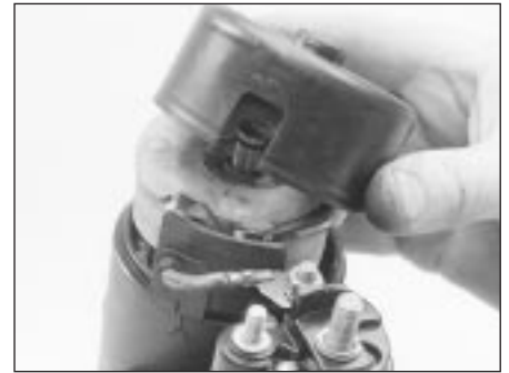
17.2C . . . and withdraw the end housing . . .
