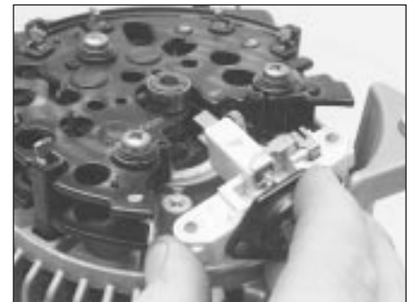
13.4 . . . then remove regulator/brush holder assembly (secured by two screws)
